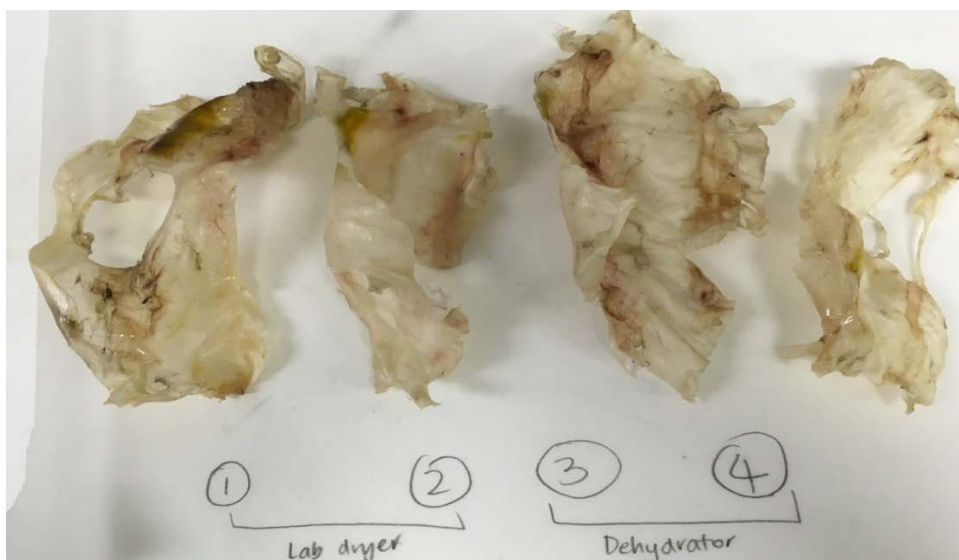
Figure 54 Air bladders dried in the convection oven (left) and Sunbeam dehydrator (right)
