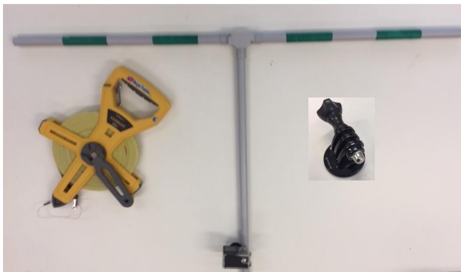
5. When filming transects, don't focus on the camera but make sure the horizontal bar of the PVC jig is held at right angles to the direction of the transect, and flat and level with the substrate.
