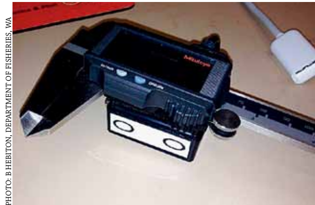
Modified vernier callipers used in the iCalliper sampling system.
