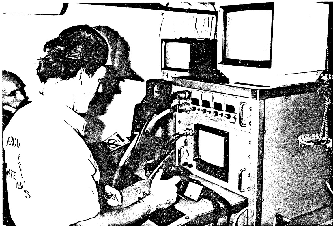
Figure 3 : The operating consoles for the ROV's. Mr. Keith Johnson is seen directing the DART with the "joystick" control aided by the video monitors.
