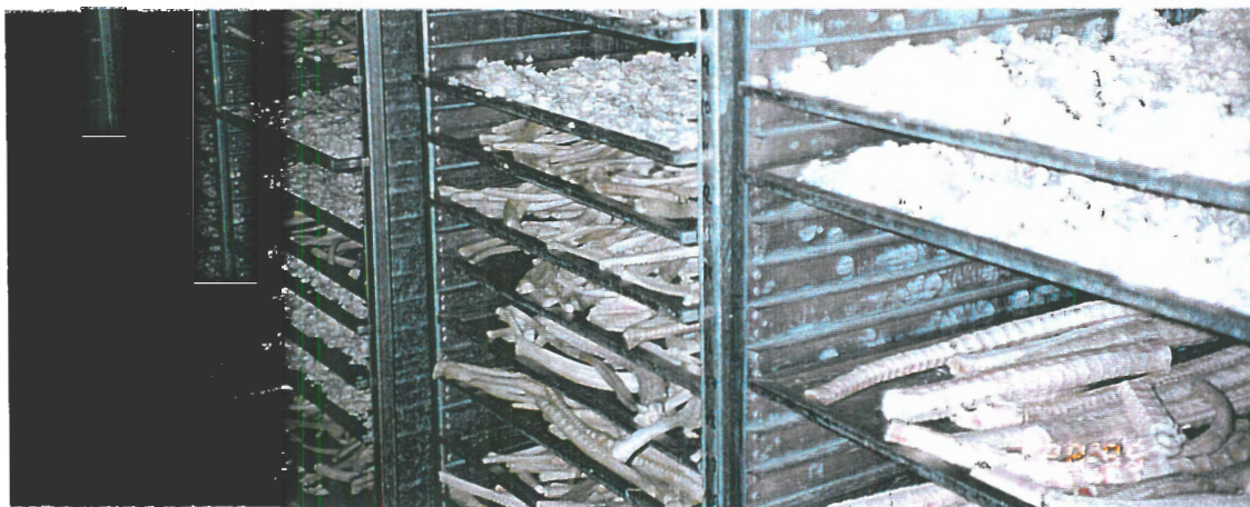
Figure 3. Cleaned shark cartilage was loaded onto metal trays and dried in a heat pump drier.
