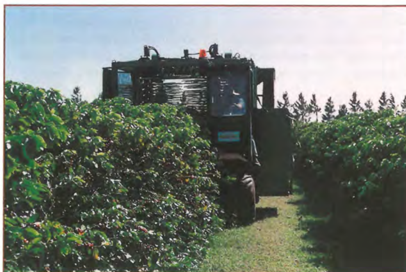
Austoft coffee harvester, showing the straddle shaker mechanism
