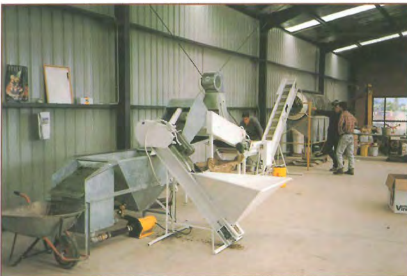
Chestnut processing operation showing small hopper, elevators, sorting table and grader
