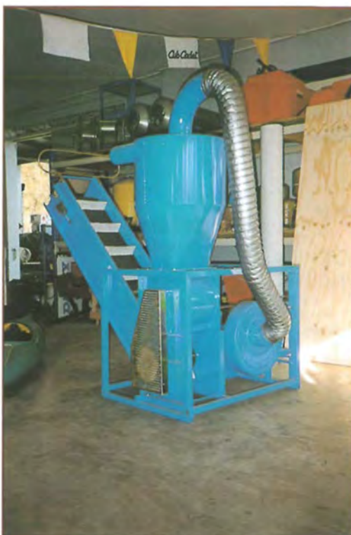
Vacuum pickup with elevator, designed to fit into a trailer
