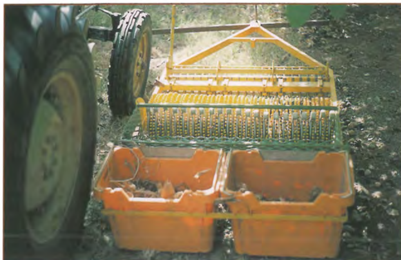
A fingerwheel harvester showing nuts being picked from the ground and collected in bins.
