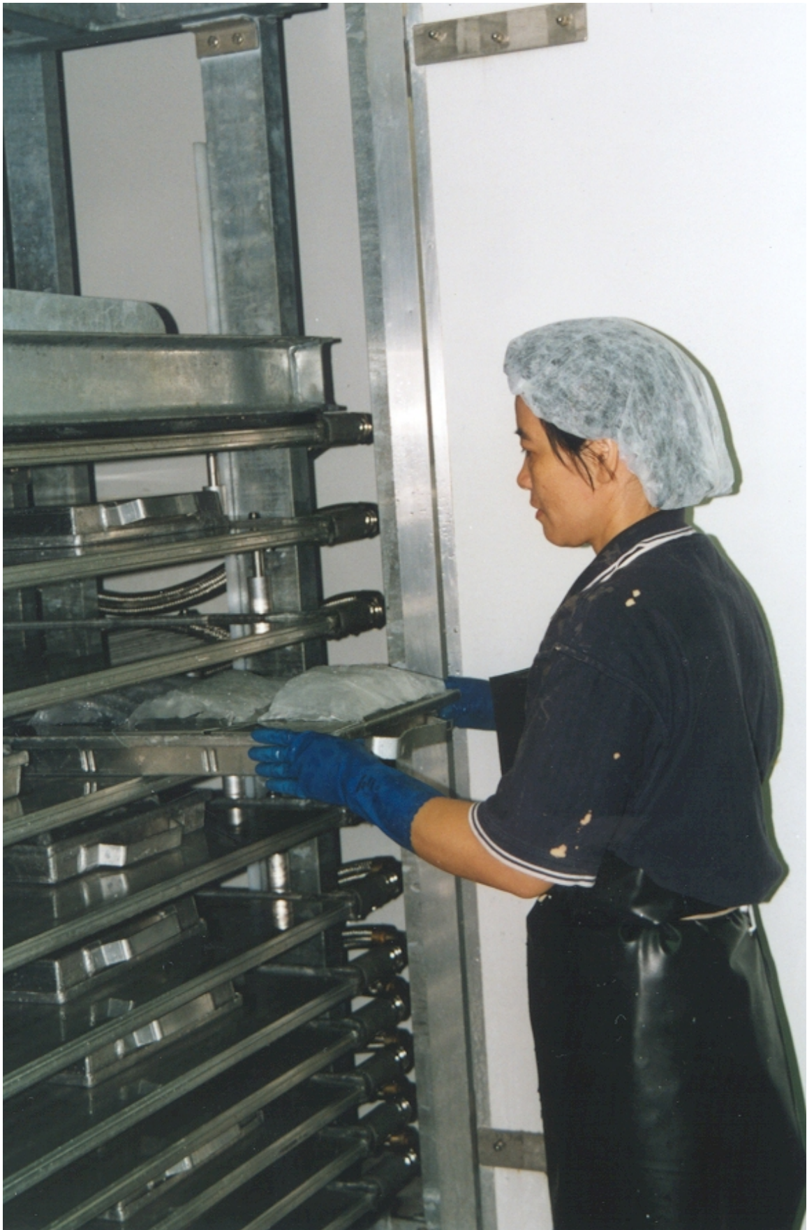
Figure 13. Placing trays containing redclaw in plate freezer.
