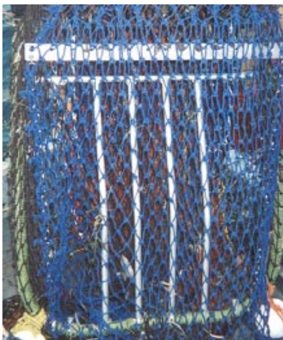
Figure 3.10 RSWN – Rectangular grid with straight vertical bars, wide bar spacing and no accelerator.
