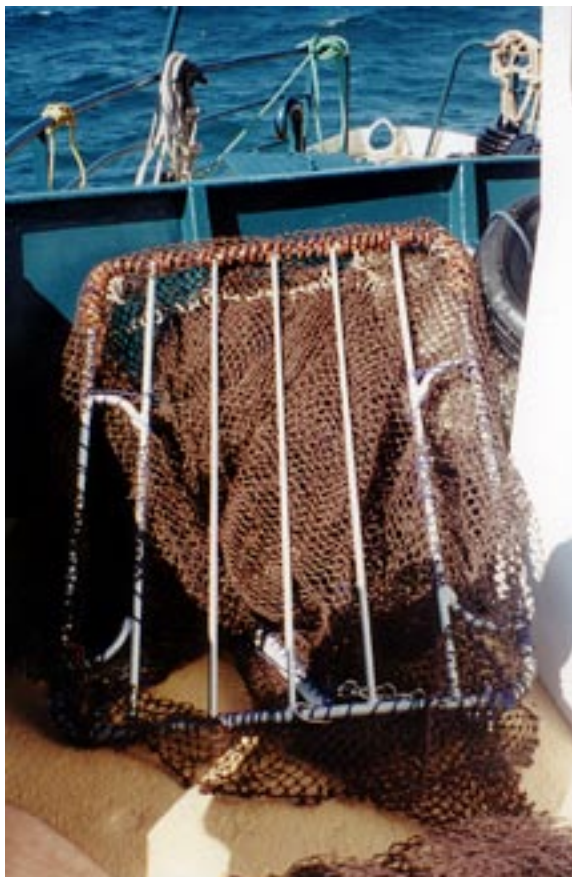
Figure 3.3 RSNN – rectangular grid with straight vertical bars with narrow spacing and no accelerator.
