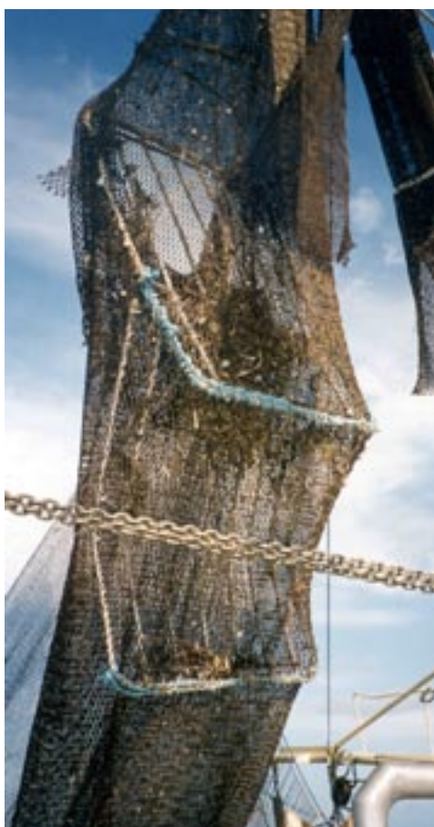
Figure 3.4 RSNN2 – Rectangular double grid, and Rectangular double grid and square mesh panel.
