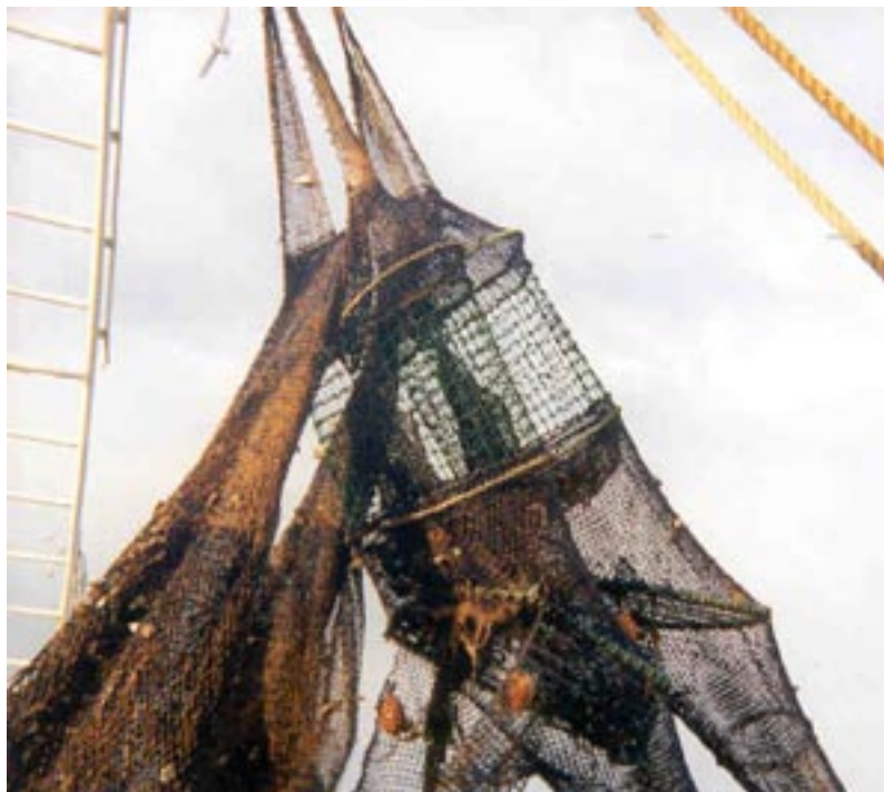
Figure 3.12 First grid type trialed in Exmouth Gulf with a radial escape section.
