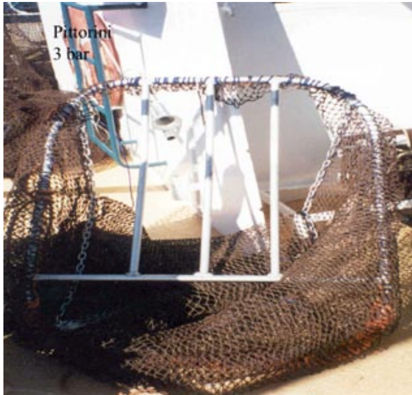
Figure 3.7 RFWN – Rectangular grid with wide bar spacing and horizontal gap with no accelerator.
