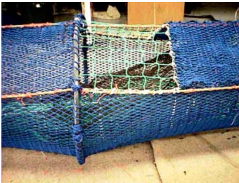
Figure 3.8 Square mesh panel and hoop set-up trialed in Shark Bay prawn fishery.
