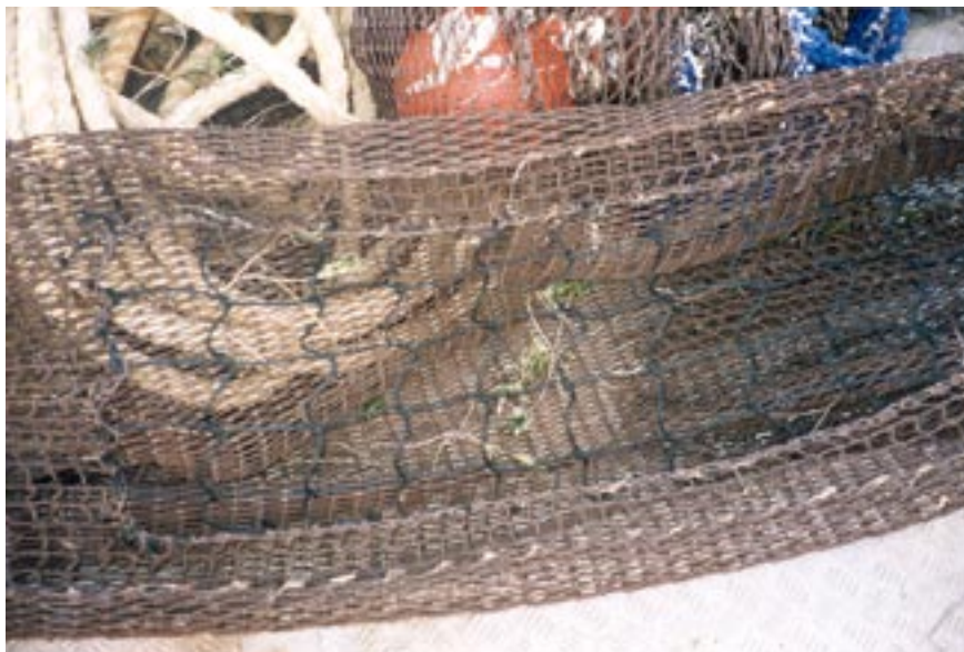
Figure 3.9 Composite square mesh panel trialed in Shark Bay prawn fishery.
