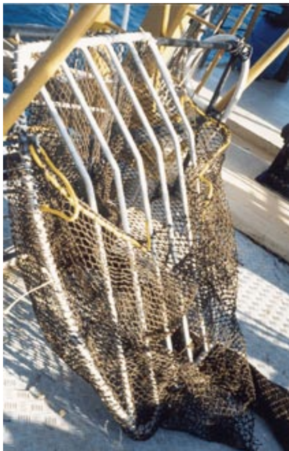
Figure 3.5 RSNA – Rectangular grid with straight vertical bars and accelerator.
