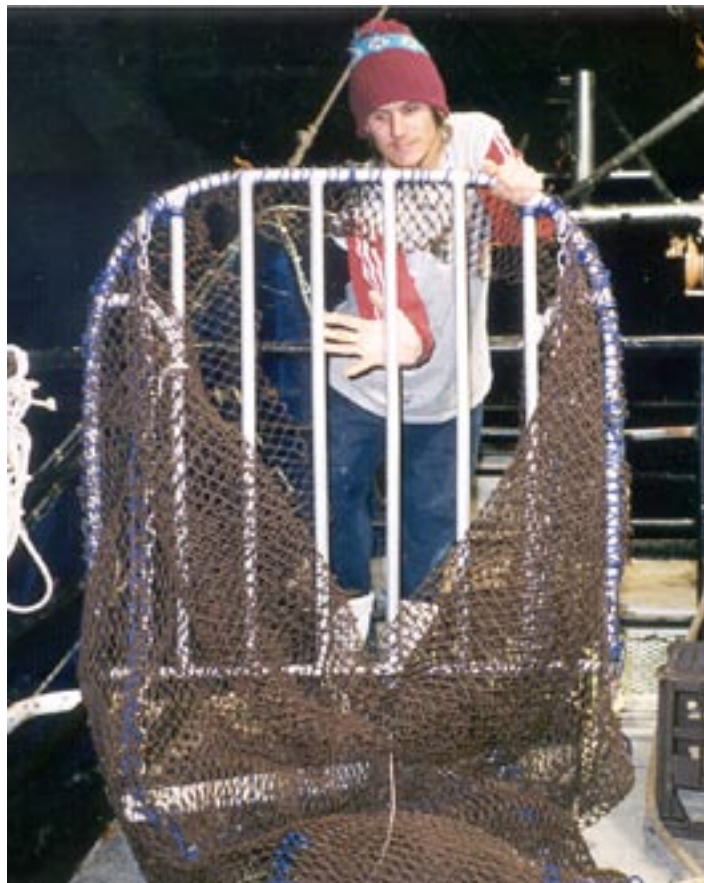
Figure 3.6 RFNN – Rectangular grid with narrow bar spacing and gap at the bottom.
