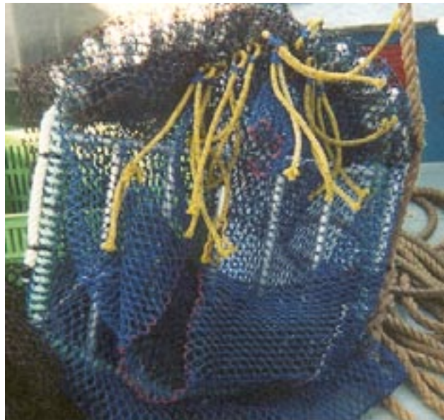
Figure 3.13 RSNN – Grid type trialed in the Exmouth Gulf prawn fishery (quad gear). Horizontal gap not effective as towed in the top-opening position.
