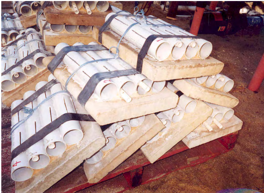
Figure 2. PVC deployment modules strapped to concrete paving bricks.
