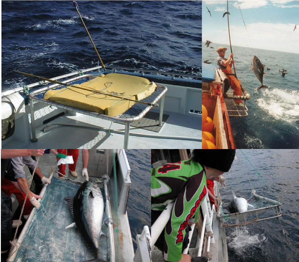
Figure 6.4. Fish landing techniques. Upper: Landing of poled fish in the Great Australia Bight onto a tagging table. Lower: Landing of southern bluefin tuna from a longline vessel using a lifting cradle. Photos by Thor Carter.
