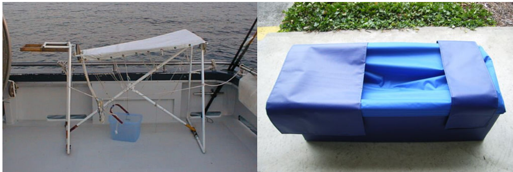
Figure 6.5. Fish tagging equipment. Left: Standard tagging cradle. Right: Portable tagging mattress designed in this project for observers in NZ and Taiwan fleets.
