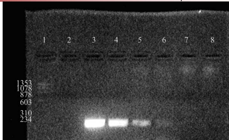
Figure 4.5 Agarose gel electrophoresis of the SSF66/SSR69 PCR products with of 1 pg of amplified Minchinia sp. DNA and varying amounts of host DNA. Samples were electrophoresed in a 2% agarose gel for 45 min at 90V. Lane 1: PhiX/HaeIII molecular weight markers. The size of each marker in base pairs is indicated to the left. Lane 2: No DNA negative control. Lane 3: Positive control. Lane 4: 200 ng of host DNA. Lane 5: 250 ng. Lane 6: 300 ng. Lane 7: 400 ng. Lane 8 500 ng.
