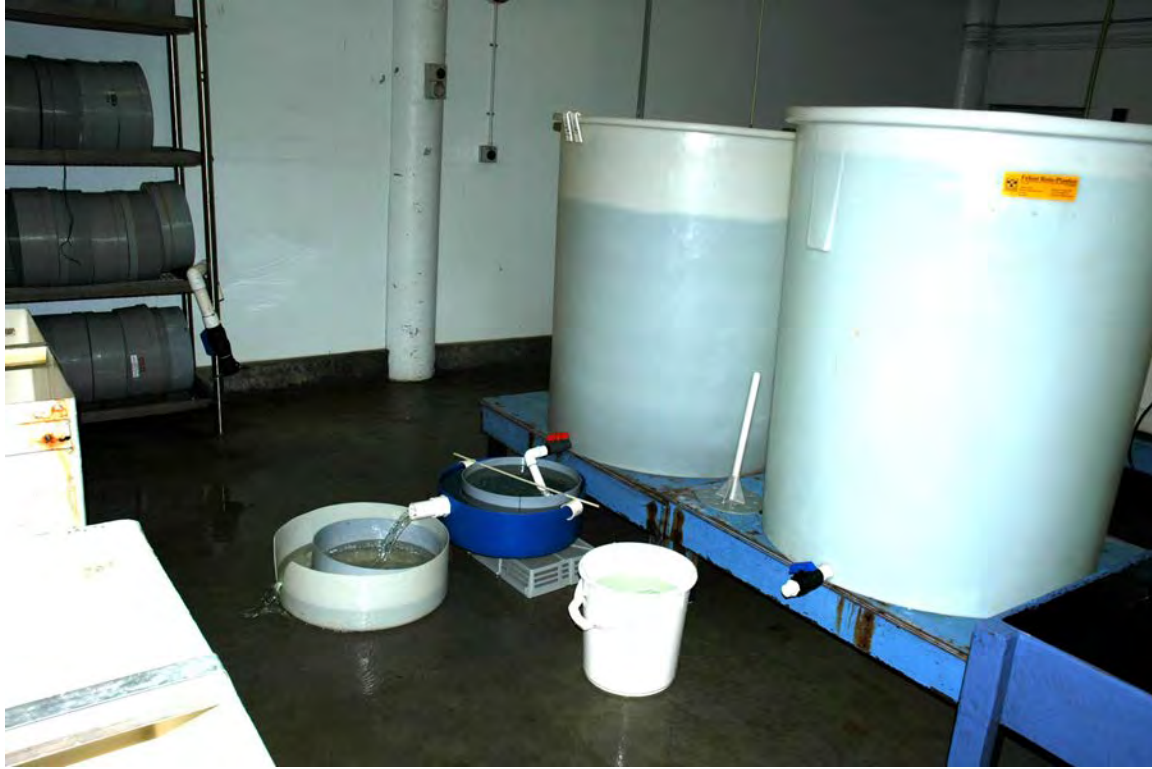
Figure 3a. Larval retention screens and apparatus used during water changes for 1000L tanks
