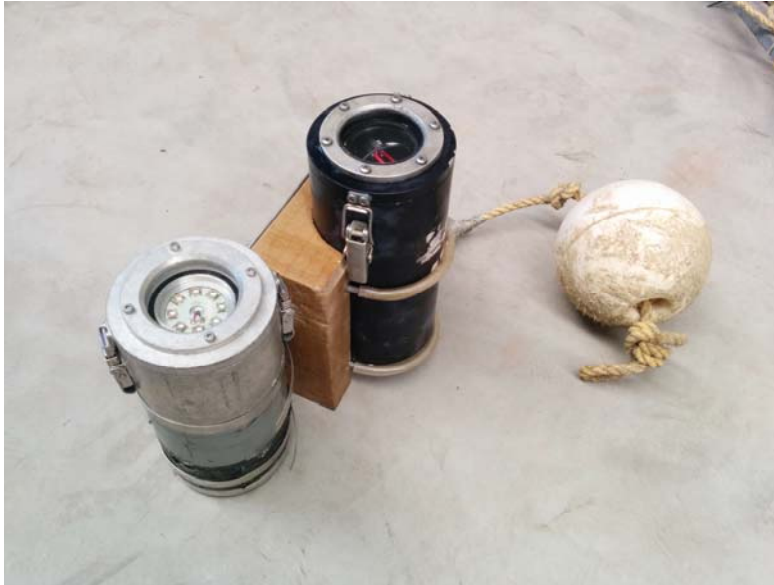
Figure 4. The underwater camera housing and float with the light housing attached.
