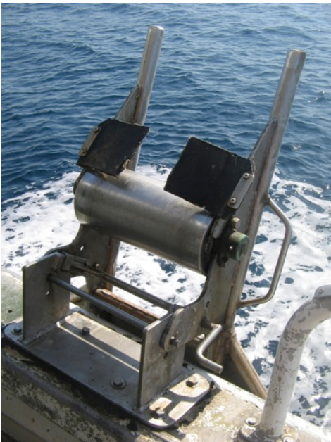
Figure 17. The floats are brought inboard through the gunwale mounted fairlead or pot tipper roller guide
