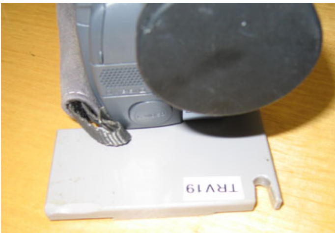
Figure 12. Inserting a camera into a housing. Note the locator slot at the front of the baseplate that locks into the lug on the housing dovetail plate. The slot should be regularly greased with silicon grease..
