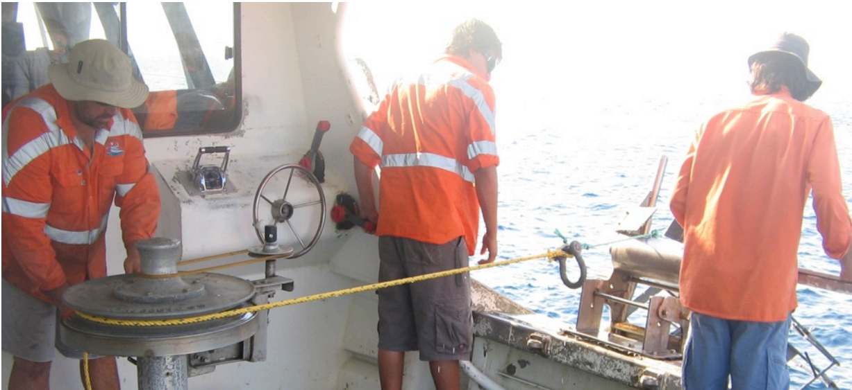
Figure 18. The rope is passed around the pot hauler winch, with one operator tailing the rope into a basket and another controlling the winch. Once the frame is at gunwale height the ballast is unloaded and the frame gently slid or lifted inboard by two people.
