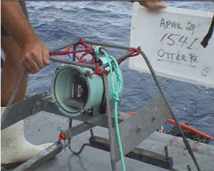
Figure 13. Site information is filmed on a “clapper board” to ensure no confusion if tape labels become lost or damaged.
