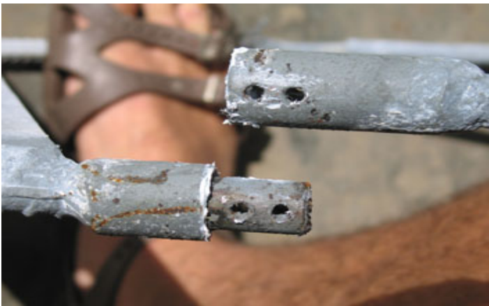
Figure 7. Male and female parts of the weak-link in each leg of the frame.
