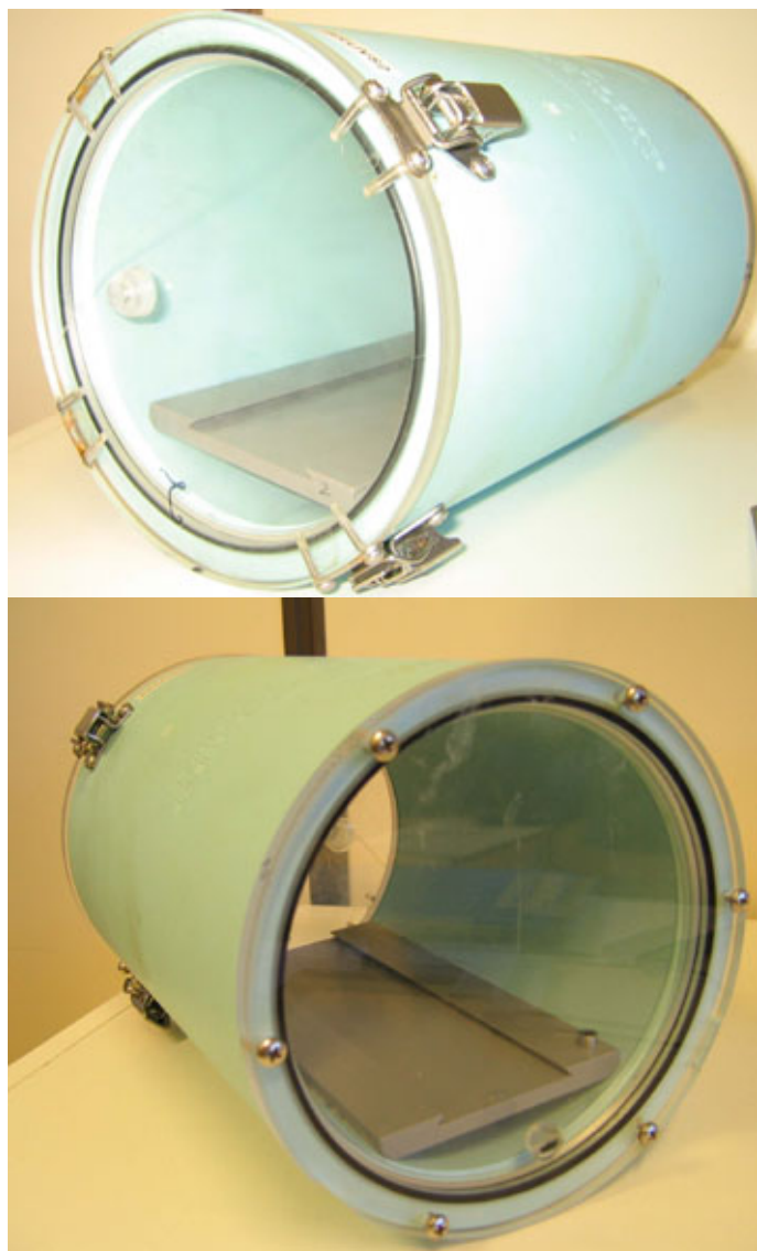
Figure 10. Camera housings showing the dovetailed plate that accepts the camera baseplate..
