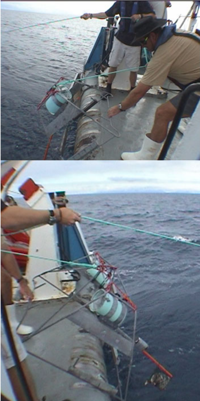
Figure 15. Ensure the BRUVS are deployed in an upright position by holding the rope immediately above the frame momentarily after the frame is slipped into the water. Dropping or tossing the BRUVS without due care causes failure and damage to cameras.
