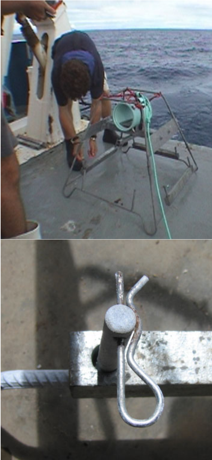
Figure 3. Removable steel ballast bars are pinned on pegs on the base of the BRUVS frame with 'R' clips. Ballast is removed and replaced every set, according to local conditions of swell and current.
