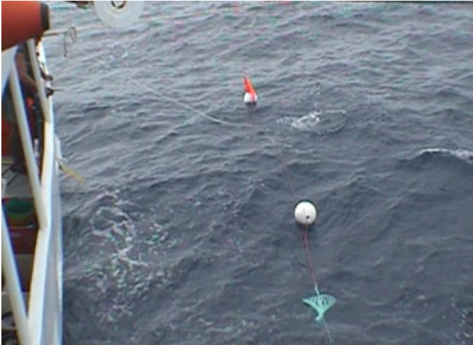
Figure 16. The vessel comes upwind or up current alongside the lay of the floats, and keeps slow forward movement. A grapple is cast between the flagpole and leader float to snag the buoy line and bring it onboard the vessel and on to the pot hauler for hauling.
