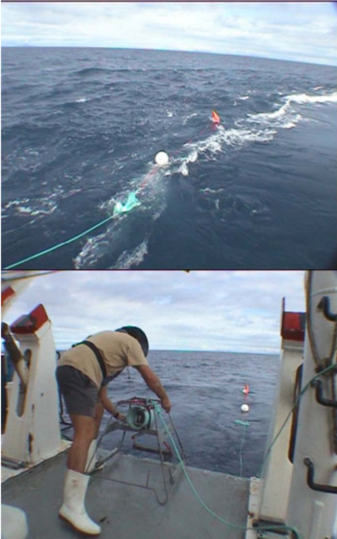
Figure 14. Floats and rope are streamed out the back of the vessel first, and locked off on a suitable strong point to await the final position of the drop. Length of ropes is twice water depth in water less than 50m deep, and 1.5 to 2 times water depth in water over 50m deep.
