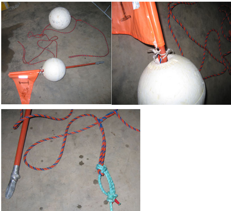
Figure 6. A float line assembly showing the 10 inch flagpole float separated from a 12 inch leader float by a 4 to 6m rope leader. This section of rope between the floats is the target for grappling during retrieval.
