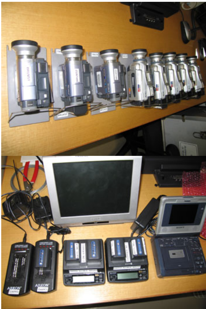
Figure 11. Sony MiniDV Cameras and a charging and playback station. Note the dovetailed baseplate attached to the cameras which interlocks with the matching plate in the camera housing.
