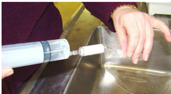
Figure 14 Sterivex unit filled by a 60mL syringe
