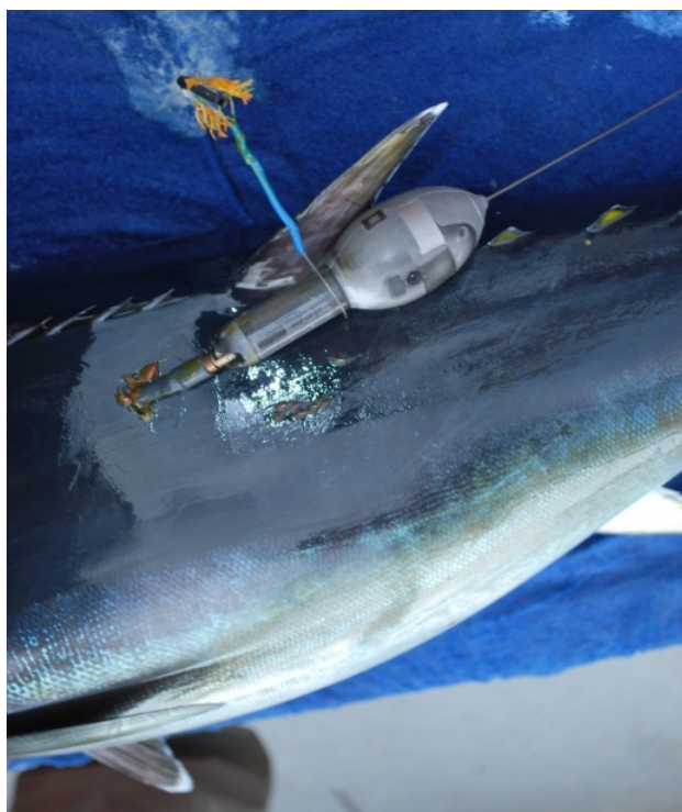
Figure 3. The primary anchor location for a 90 cm fork length Southern Bluefin Tuna. Note the tagging site is anterior to the pterygiophores. The secondary anchor (shown with blue heat shrink cover) is not yet inserted, but its position allows for insertion into the pterygiophore complex of the second dorsal fin. Photo credit: Jarrod Day.
