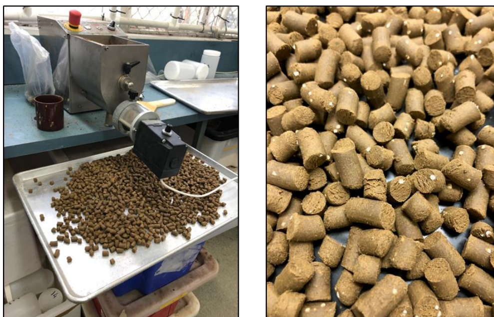
Figure 1: Pellets made with Dolly pasta maker for palatability and efficacy trials. Note white PZQ beads in the right hand photo.
