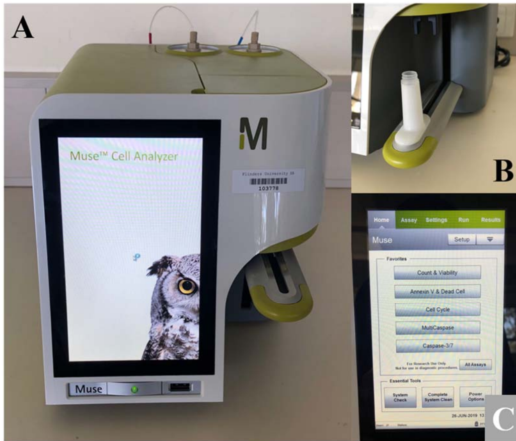
Figure 2.1 Overview of the Merck Muse Cell Analyser, highlighting (A) physical bench top size of the machine, (B) the sample loading arm and (C) the touch screen interface.
