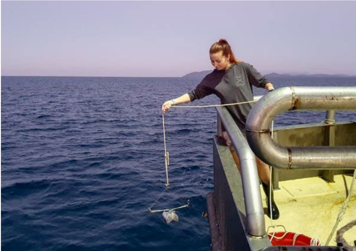
Figure 21. Samples of sediment and eDNA were collected with a sediment grab at each site, as well as recordings of depth, temperature and salinity readings taken using a CTD probe before sites were trawled so that sediment was undisturbed by trawl gear prior to sampling.
